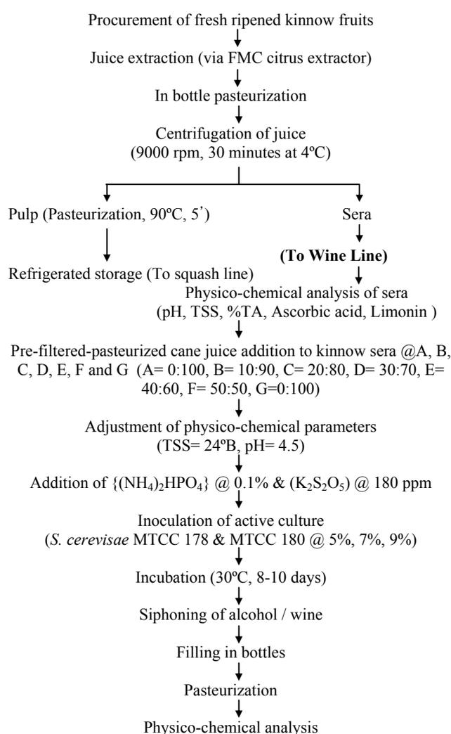
**FIGURE 1. Flow diagram for the preparation of pure and blended kinnow-cane wine.**
